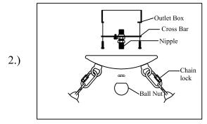
Step.2: Attach cross bar to outlet box. Secure canopy to cross bar by threading ball nut onto nipple. Hang fixture (D) and use chain lock to connect chain to canopy (B).
