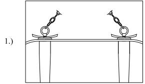
Step.1:Install top loops (A) and attach desired amount of chains to loops to achieve desired mounting height. Thread wire through every 3rd loop of chain. Place Candle Covers (C) over sockets.
